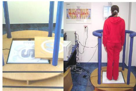
This posturographic system has allowed a real-time display of results and allowed detection of minor changes in subjects' ability to maintain balance and adjust the static and dynamic conditions both in the presence and in the absence of visual information. There were highlighted two diagrams for the two planes of movement (antero-posterior and medio-lateral).
